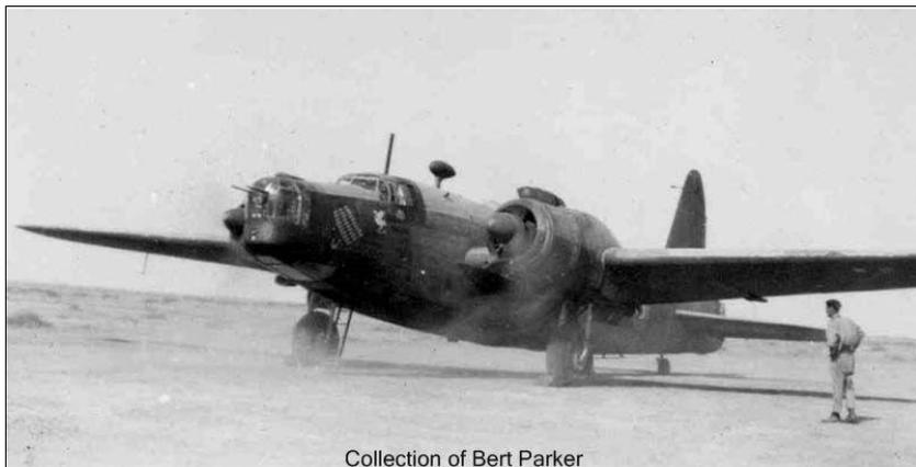
Hercules engines. These air cooled radial engines were much preferred over the liquid cooled Merlin engines, in Wellington II's and Halifaxes that were also used in this theatre, which would often overheat and were more affected by dusty conditions. The tropicalized Wellington Mark X were also slightly lighter than the Mark III with an empty weight of 26,325 lbs and when
